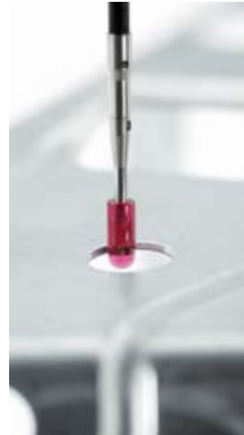
Cylinder styli e.g. for measurement of metal sheets
