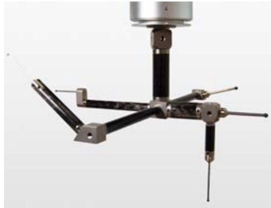
A complex stylus configuration with multiple components
