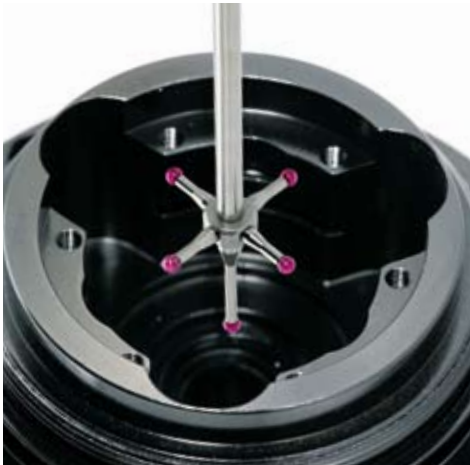
Measuring a complex interior contour
