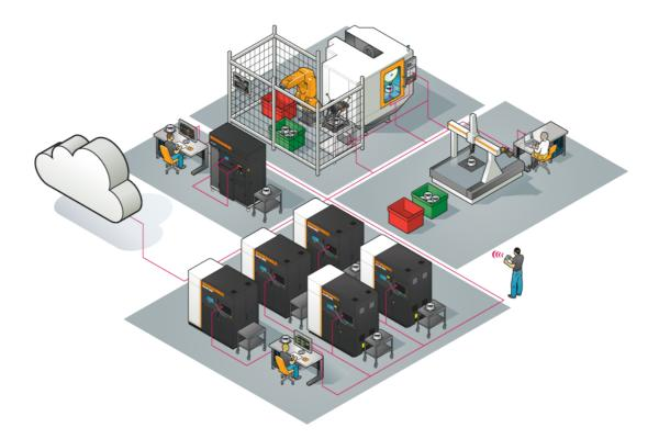
As well as supporting standard connection interfaces such as MTConnect, Renishaw Central is built as an API that can be directly consumed into existing ERP and MES software.
