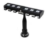
Based on the industry standard range of MCR20 rack systems, TCR20 securely stores modules for rapid automatic changing, protecting mating surfaces from any airborne contaminants within the working envelope of the machine.
