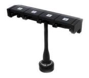
The SCR600 is a passive stylus change rack and so it requires no electrical connections. It is protected from overtravel (in the probe entry direction) by a mechanism in the base which can be manually reset.
