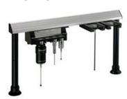
The MRS modular rack system provides a platform for Renishaw probe and stylus changing racks. It consists of a rail (400 mm, 600 mm or 1000 mm long) that holds the probe or stylus changers, and interconnecting legs of selectable lengths that allow clearance for long styli and extension bars.
