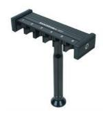
The MAP stand can be mounted directly onto the table of a CMM (or any suitable surface) using the appropriate socket head bolt which is passed through the centre of the base.
